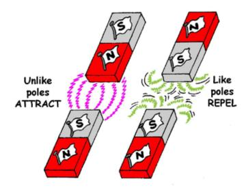
Magnetic forces like this also appear whenever there is a flow (current) of electricity, an effect which is used to make the electromagnets that pick up old cars in scrap yards. The stronger the current, the stronger the force – so, by measuring the force it is possible to determine what the current must be. This is the basis of the definition of the ampere, the unit of current.
